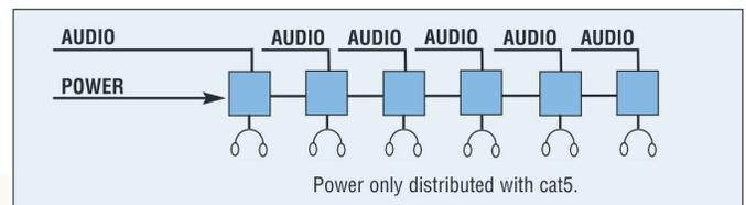
Any combination of the installations above is possible, using cat5 to distribute power and audio to some GuestPods, with other units receiving power only via cat5 + local audio via the GuestPod TRS input jacks.
