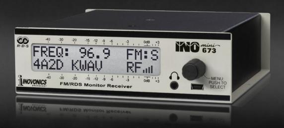
The INOmini 673 is Inovonics' second-generation, small form-factor FM broadcast monitor for professional applications. A sensitive and selective off-air receiver for standard analog-FM broadcasts, it has application as a 'confidence monitor' or as a rebroadcast receiver in FM translator service. The 673 decodes and displays the most important data from RDS/RBDS data groups as well.
