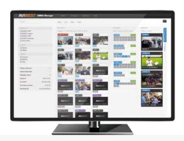
The MANAGER is a powerful application that enables broadcasters and video professionals to monitor and manage an entire live video contribution system including AVIWEST transmitters and encoders, smartphones using the MOJOPRO, and STREAMHUB transceivers, as well as third parties equipment through its RESTfull API.
