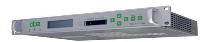
ABE "IRD1001/AW" is an Integrated Receiver Decoder that demodulates digital QPSK and 8PSK signals according to DVB-S and DVB-S2 specifications (for Broadcasting applications) in the "L band" (the standard IF output of an LNB – Low Noise Block downconverter) and decode the selected video / audio program according to MPEG-2 (4:2:0 – MP@ML) analog outputs. It also support Conditional Access.
